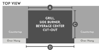
D = Notch out width of countertop overhang should be cut back to the cabinet base to allow appliance to sit flush with base.
