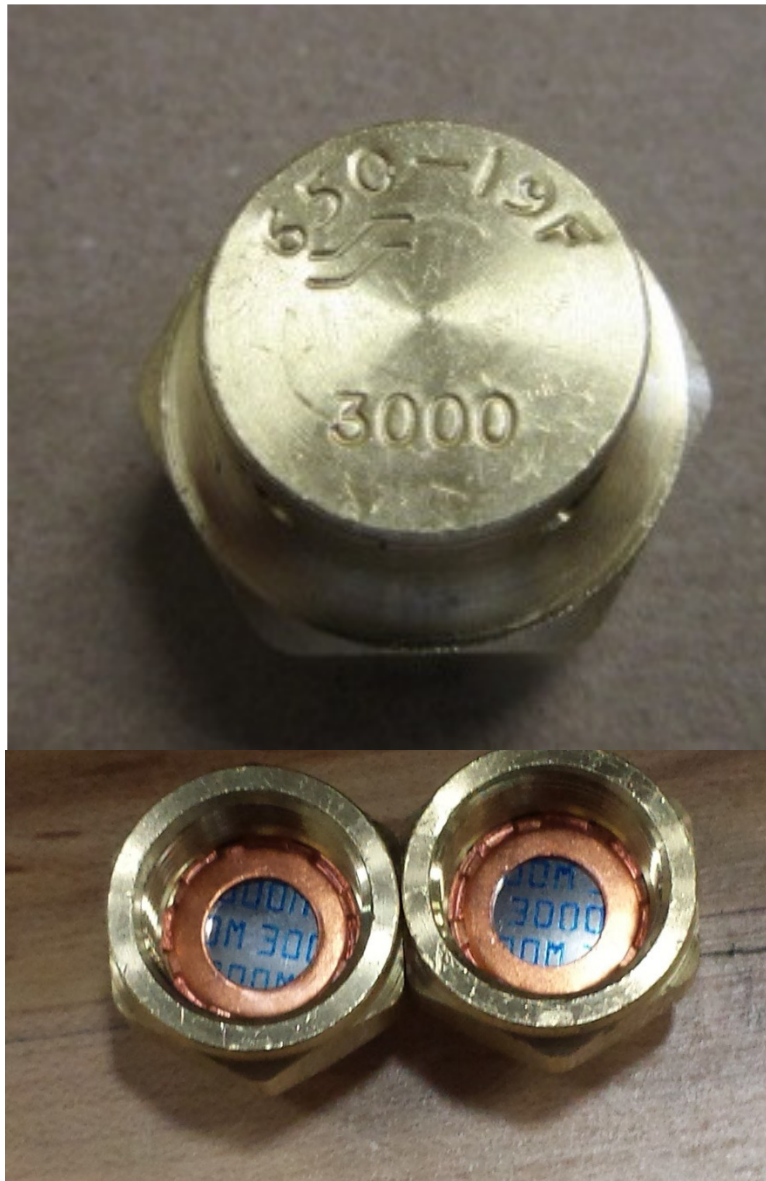
Figure 1 (650-19F9-28, burst disk correctly rated for 3000 psig)
