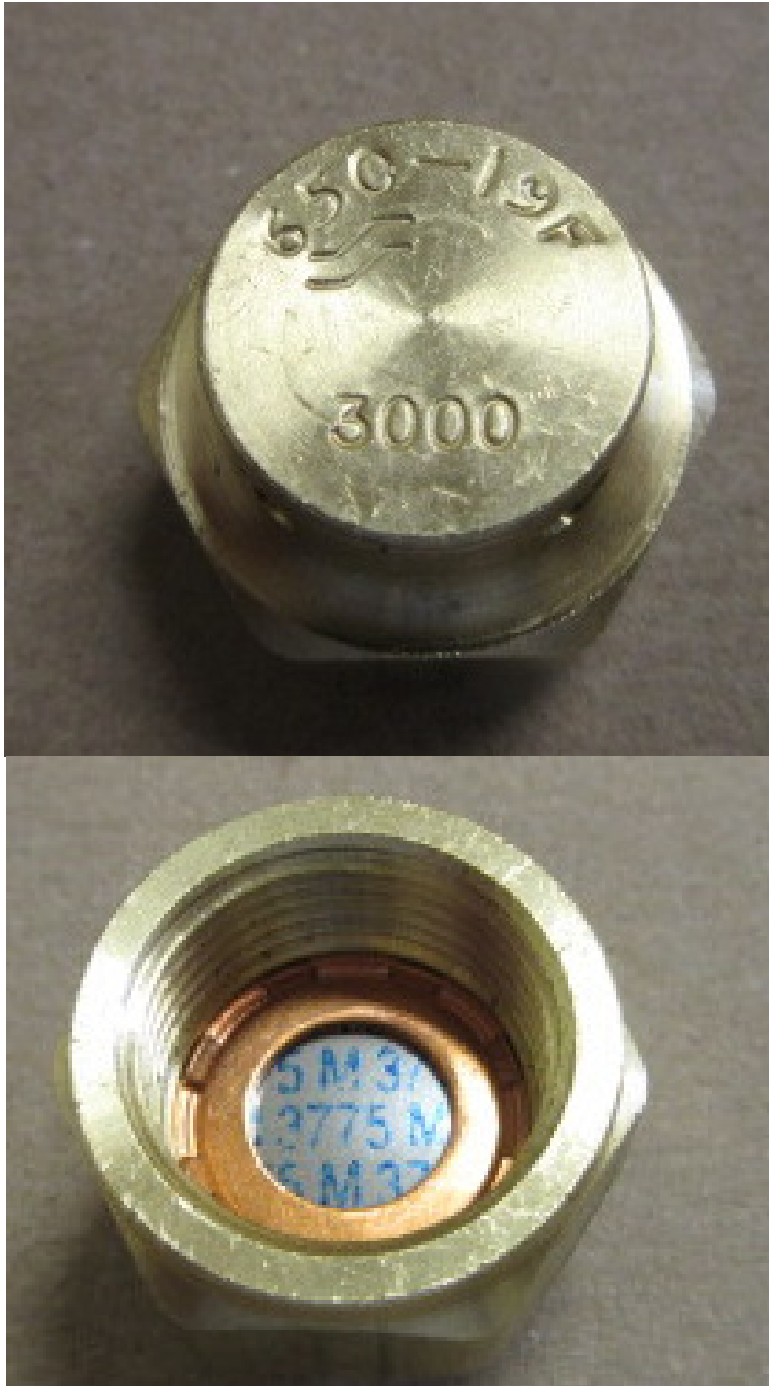
Figure 2 (650-19F9-28, burst disk incorrectly rated for 3775 psig)
