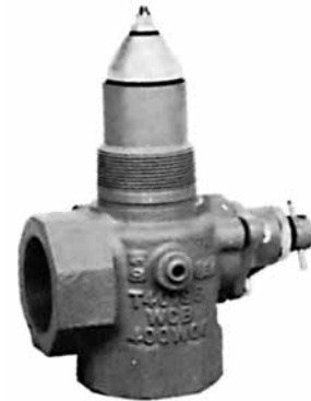
C471 C471 internal valve with two outlets, bottom and side. The side outlet permits installing horizontal piping immediately adjacent to the tank. The C471 is used primarily on bobtails and transports.
